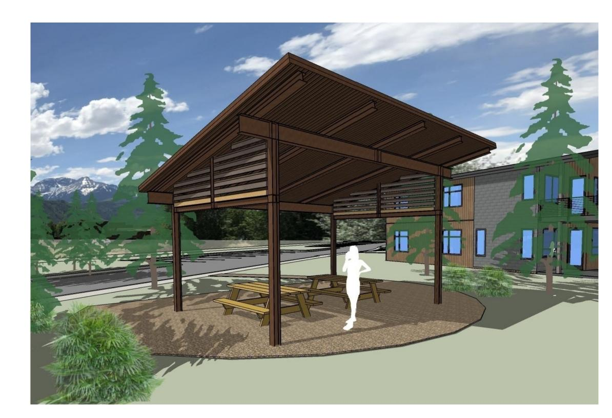
SPECIFICATION: STRUCTURE: STEEL I-BEAM STRUCTURAL SECTION NATURAL FINISH ROOFING: CORRUGATED PRE-FINISHED SIMULATED RUST INFILL PANELS: 2x CEDAR
