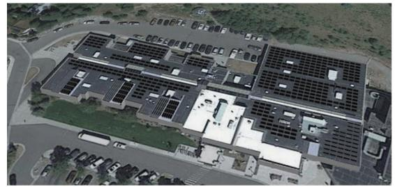
This microgrid project includes solar for load offset and batteries for both resiliency and self-consumption/demand charge reduction. The project economics depends on the savings afforded by the batteries being able to shift delivery of the daytime solar and clip peak demand. The batteries then serve as back up for critical loads during a power outage. This system architecture is becoming quite common, and our policies enable the approach.
