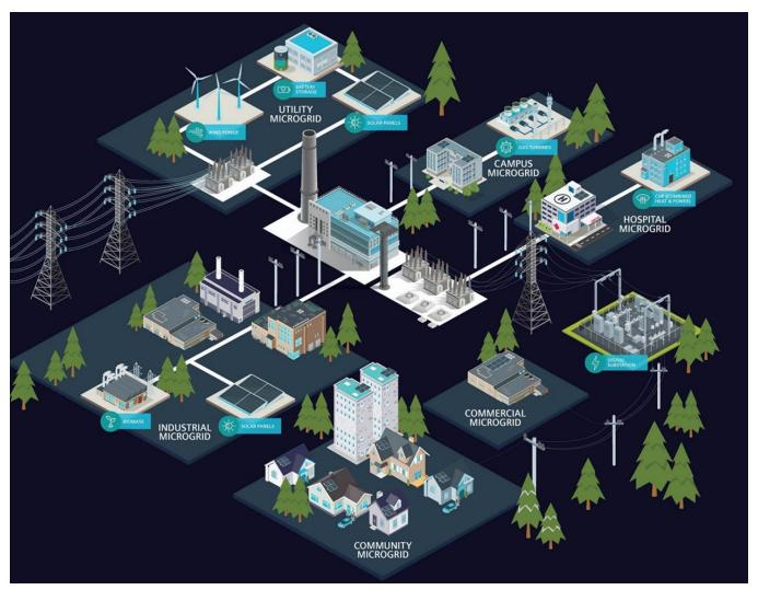
Microgrids include multiple power generating sources with local energy storage that can "island from the grid" during a power outage.
