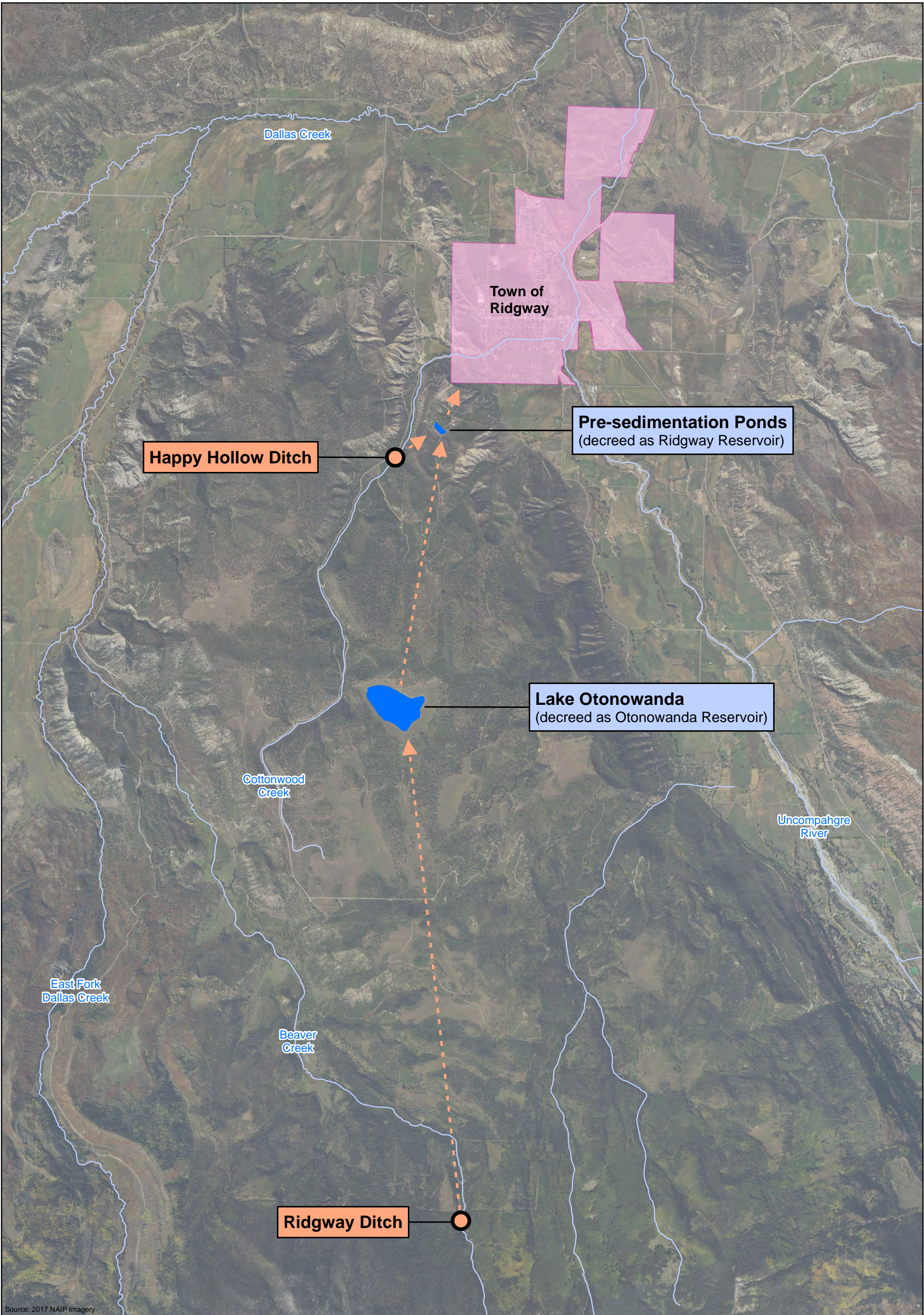
Figure 2 Schematic of the Town of Ridgway's Water Supply System
