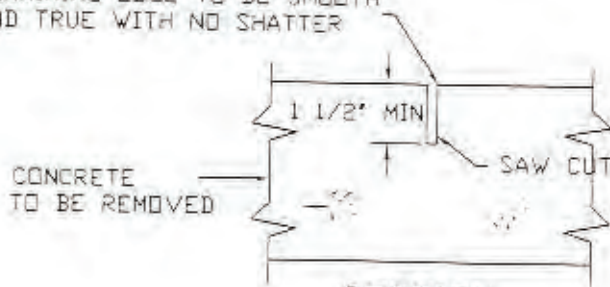
SECTION SHOWING CUT
