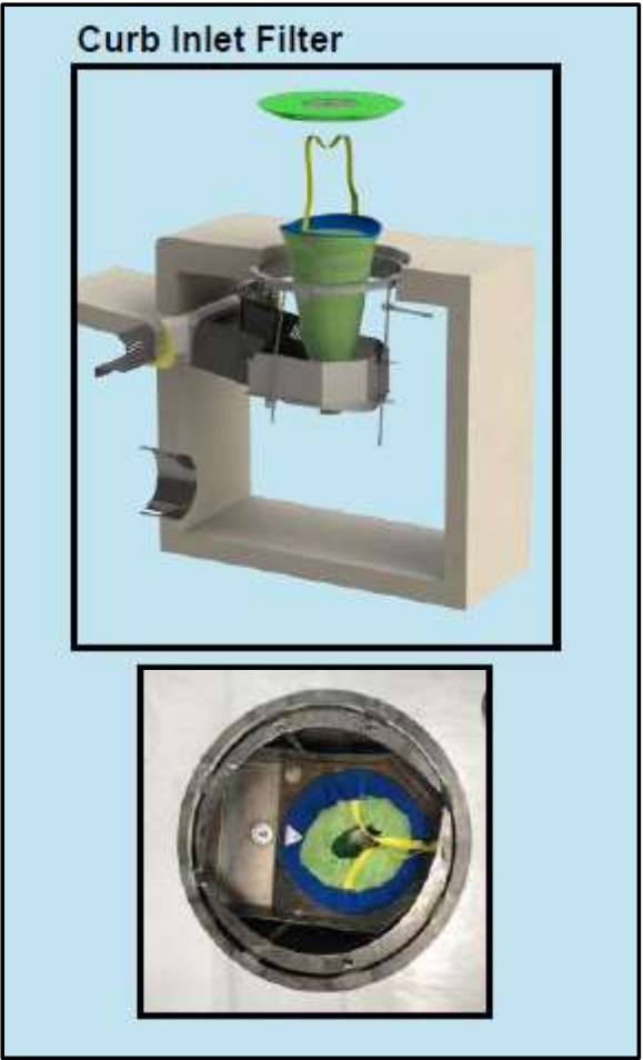
Figure 4-10. Example SH 62 Inlet BMP (Frog Creek’s Gutter Bin)
