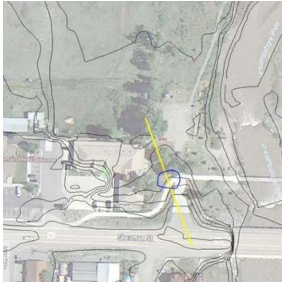
Figure 3-9. Preliminary routing of piped stormwater to Rollins Park. Routing to the park would come with significant costs.
