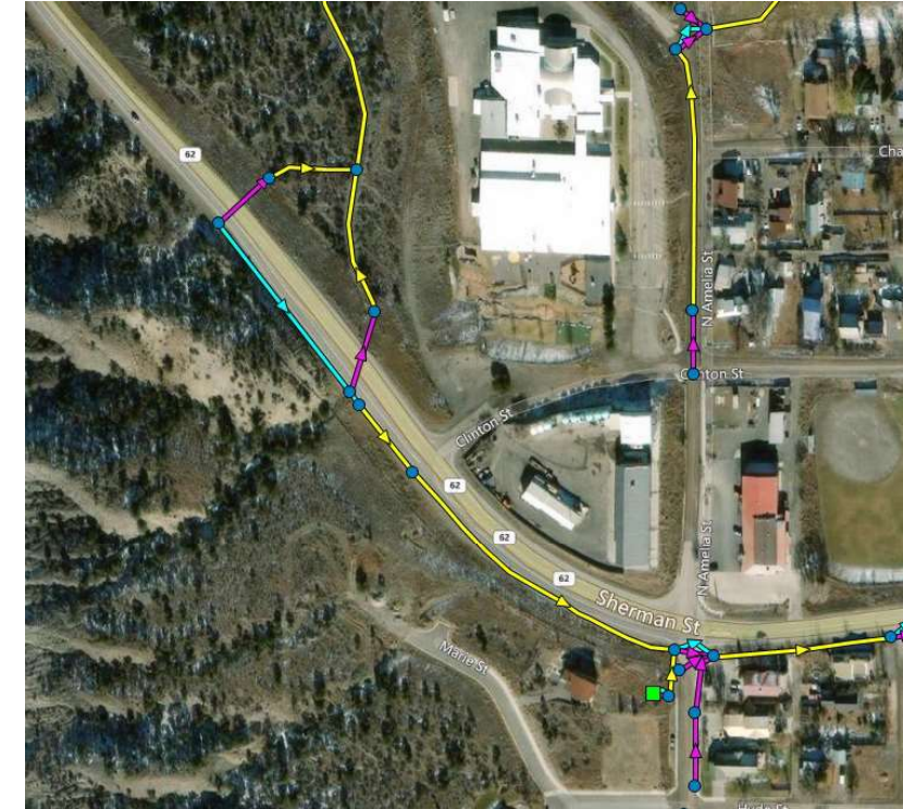
Figure 2-11. Stormwater flow paths at SH 62 west of Amelia St.
