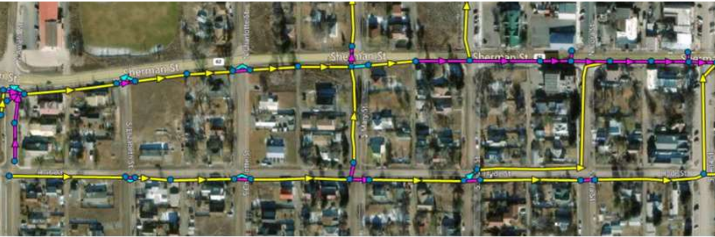
Figure 2-12. Stormwater flow paths along Hyde St.
