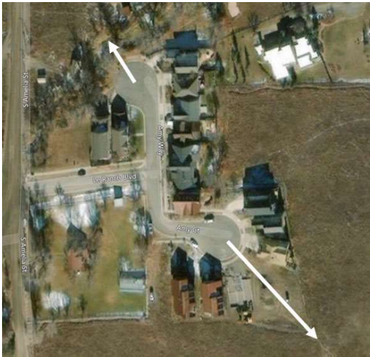
Figure 2-8. Stormwater flow paths from Amy Way and Amy Court
