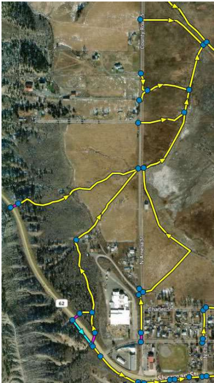
Figure 2-15. Stormwater flow paths between SH 62, CR 5, and the upper reach of Big Ditch
