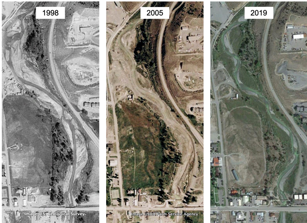
Figure 6. Channel evolution downtown, pre/post restoration and current conditions.
